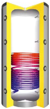
HAPSR 500 - 1,000 Buffer storage tank made of steel S235 with 1 heat exchanger, operating pressure 3 bar, max. operating temperature 95°
